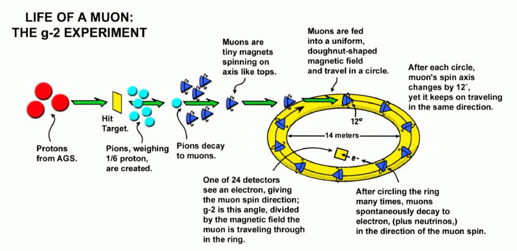
Coupling of muon to magnetic field :  $\mu - \mu - \gamma$  coupling
