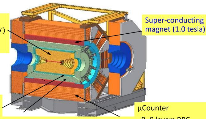
$\sigma E/VE(^{0}/_{0}) = 2.5 \% (1 \text{ GeV})$ EMC: (CsI)
