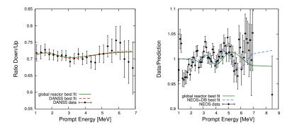
DANSS: relative spectra @ detector locations with L = 10.7 and 12.7 m
