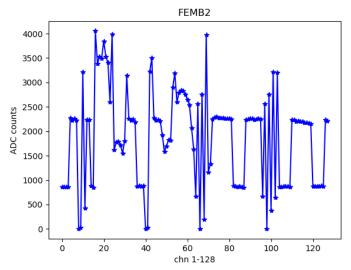
We met this issue before in BU firmware. Data are not aligned. It turns out to be the configuration issue.
