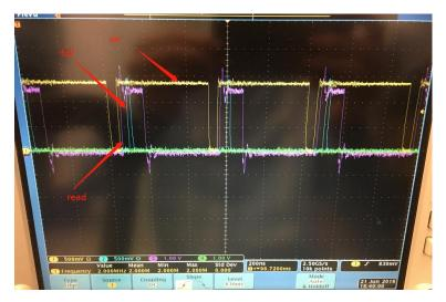
Now the fifo write enable signal becomes normal and we get the ADC data, but the full signal should not appear since read process is more faster than write process.
