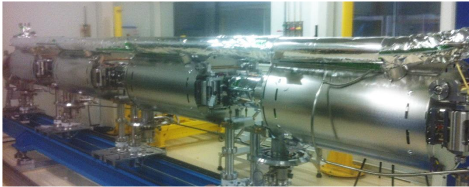
Horizontal test cryostat SATHORI
