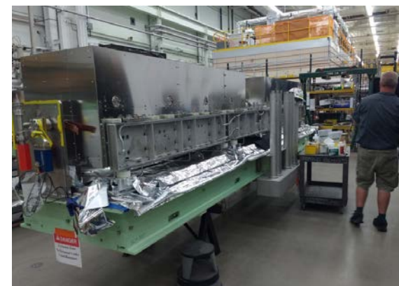
PC-Permalloy magnetic shield on a 0.53HWR cryomodule
