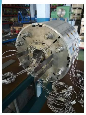
mock-ups to measure mechanical parameters, validate calculations and train with the B&K assembly process
