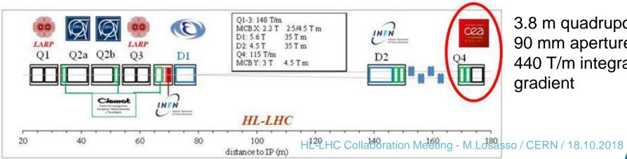
3.8 m quadrupole 90 mm aperture 440 T/m integrated gradient
