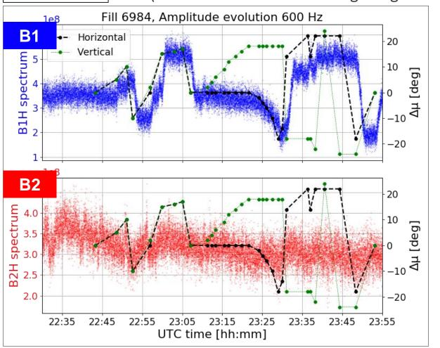
Changing the phase advance between IP1 & IP5 in B1 affects the amplitude evolution of the harmonics in B1.
