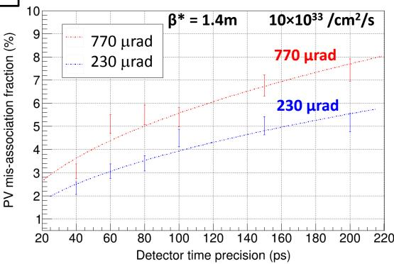
Change in **crossing angles** leads to different performance (in terms of PV reconstruction, and PV-matching for long-lived particles)
