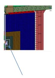
Innermost part of the ECAL, to be replaced in LS3 because of radiation damage
