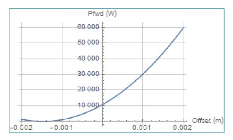
HL-LHC case. Power required with 3 MV/cavity. With -1.5 mm offset the power actually goes to zero, as the beam-induced crabbing voltage equals the demanded 3 MV. If the offset is +1.5 mm we need about 45 kW.
