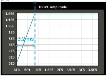
Pulsing the CC RF in the SPS: Linear drive ramp lasting for 3.2 ms (bottom).
