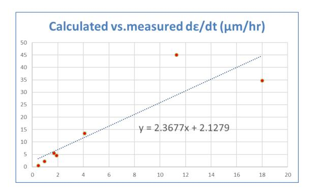
Calculated (eq. slide 5 using measured spectra) vs. measured (Wire Scan) during the coasts with different noise levels. The calculations over-estimate the growth by factor 2-3. With CC off the growth rate is around 0.4  $\mu m/hr$ . Wire scan measurements by L. Carver.
