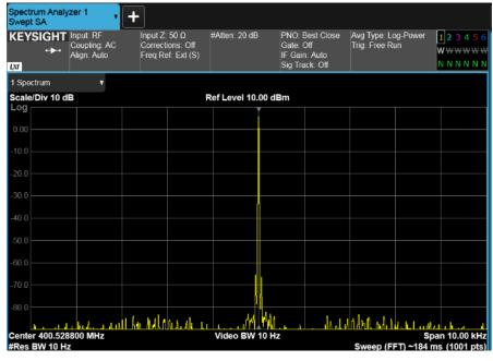
Spectrum of ANT (centre freq. 400.528800 MHz, 26 GeV, 10 kHz span).
