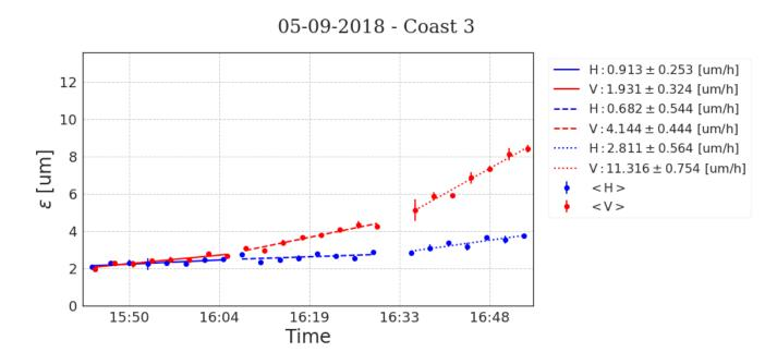
Measured growth of the horizontal emittance in blue (up to 2.8  $\mu$ m/h for the largest excitation, to be compared to the vertical 11.3  $\mu$ m/h in red) while the CC kicks are strictly vertical.
