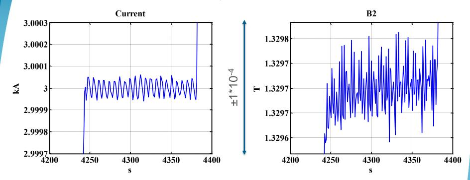
During plateaus, at field levels in the range where the flux jumps have maximum amplitude, we see noise on the measured field with amplitude <1\*10<sup>-4</sup> (limited by measurement precision).
