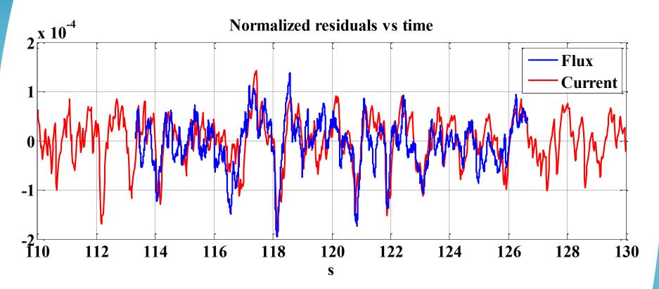
During ramps, in the field range where the flux jumps have maximum amplitude, we measure a "noise" with amplitude ~1\*10<sup>-4</sup> on both current and field.
