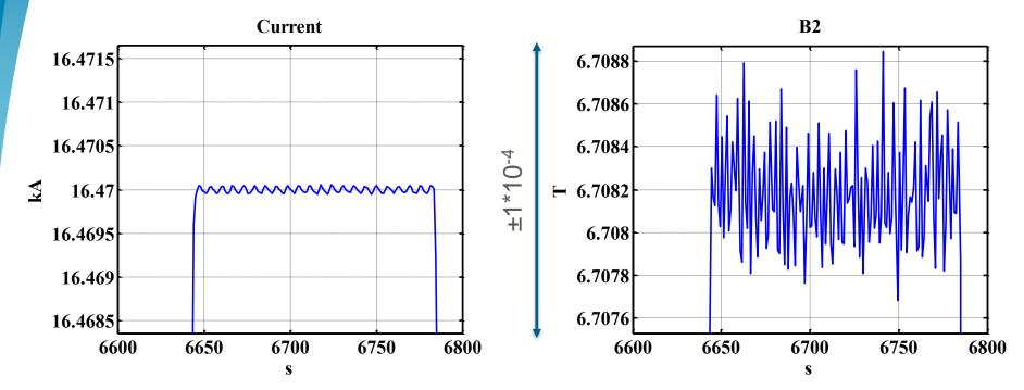
During plateaus at nominal field, the noise on the field has amplitude <1\*10<sup>-4</sup> (limited by measurement precision).
