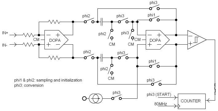
Wilkinson ADC: differential amplifier and comparator Amplifier topology the same as for integrator (open loop gain 90dB) but bandwidth limited to 60MHz.
