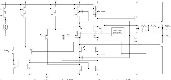
Fully-differential two-stages amplifier with cascode Miller compensation and class AB output.
