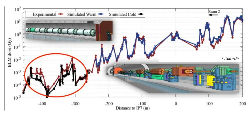
BLM signal benchmark in IR7 quench test
