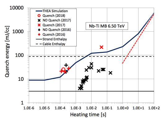
Good agreement between multi-strand 1D model of stability and results derived from the quench tests in the LHC!
