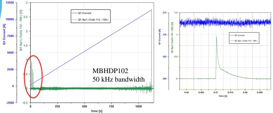
• The amplitude and duration of these spikes is larger wrt the baseline protection settings (100 mV, 10 ms).
