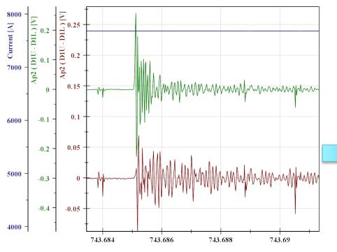
A Median filter of 50 us could be a solution (2-3 samples with a sampling rate of 50 kHz) Moving average filter of 10 samples Both easy to implement on the FPGA
