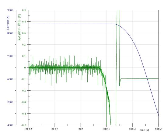
Emulation of the Logics for the Quench Detection (implemented on the FPGA)
