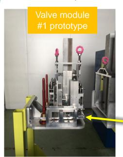
Handling tests on real mock-up (CMS type) with final module supports and dummy loads (vacuum instrumentation) ongoing under the coordination of WP8
