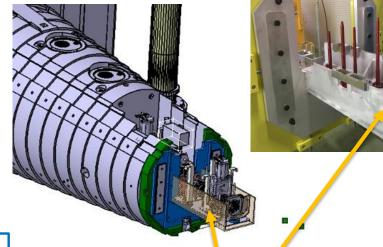
New beam pipe support on FIN (CMS): designed to accommodate the future new HL-LHC VAX
