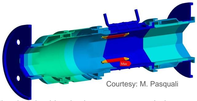
Cooling inspired by the beam screen solution Electrodes **5** K above beam screen's temperature
