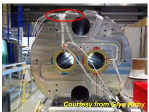
Fig.3 Front view of CCT prototype exit leads
