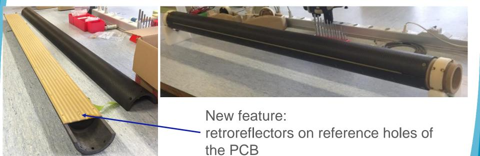
Accurate knowledge of the coil position (integral field, magnetic length, longitudinal center)
