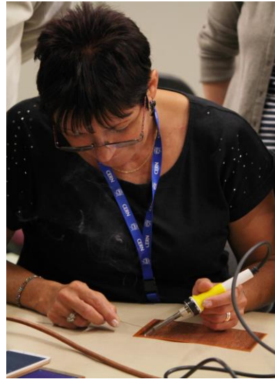
Soldering the electronics boards for the chambers
