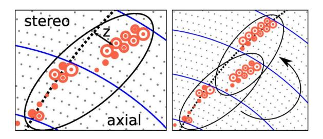
Cellular automaton with vertices from a pair of segments in axial+stereo layers. Segments that share common segment form edges. Weights based on Riemann fit in x-y and linear fit in s-z space.
