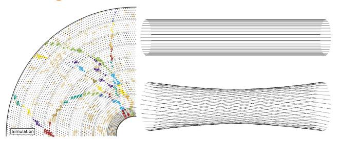
CDC consists of 56 layers, arranged in superlayers of axial and stereo wire orientation. Global track finding stats in x-y, followed by s-z reconstruction. Local track finding starts with building segments in superlayers, and then connecting them
