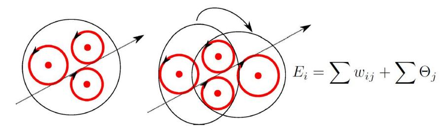
Cellular automaton with vertices associated to triplets of hits with and a linear track-element trajectory. Edges are from neighboring triplets, sharing two hits. Weights are based on a quality of the common fit
