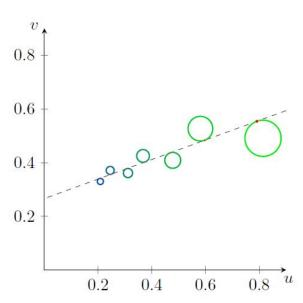
Conformal map to transform circular in x-y trajectories to straight lines. Drift circles transform to circles. Track finding reduces to finding common tangent to the set of circles.
