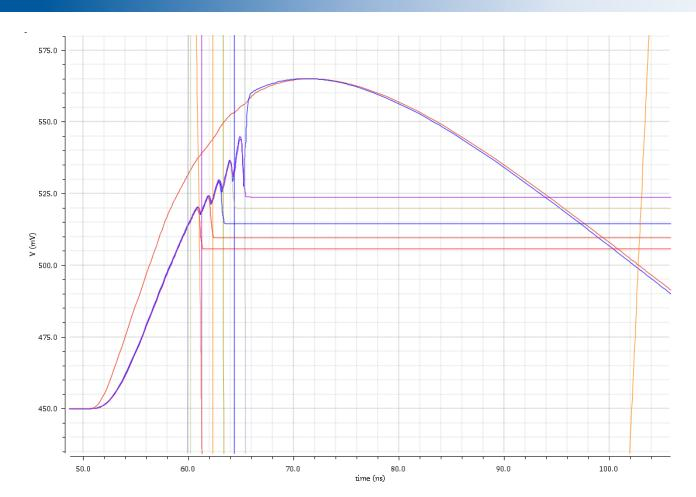
Input charge 2k - Power consumption =  $25.72 \mu W$
