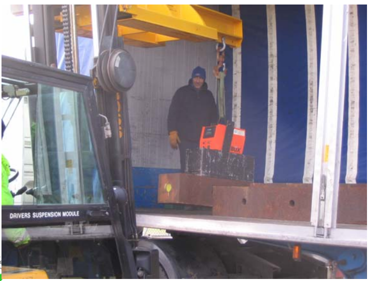
Unloading steel with electromagnet
