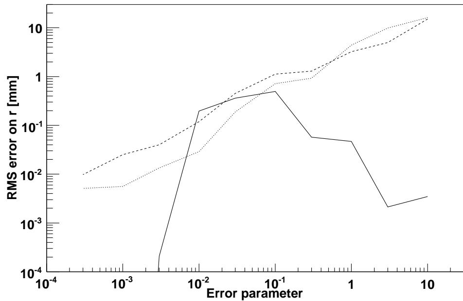
Fig. 1: Error on position vs tracking parameters: (full) deltaOneStep (dashed) missDistance (dotted) deltaIntersection
