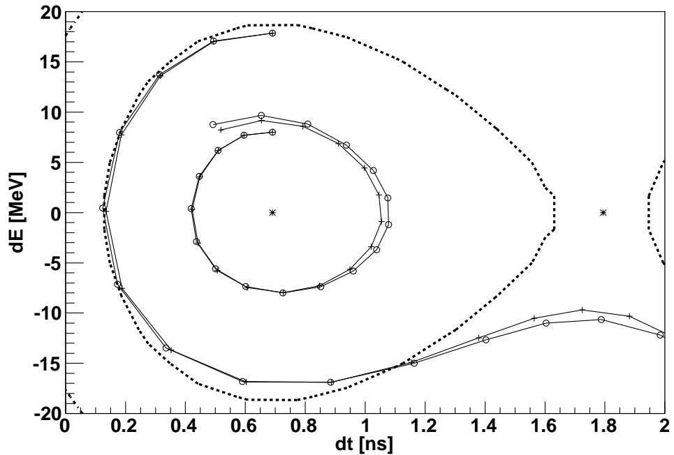
Fig. 3: Muons traversing the RF bucket (o) using RF field maps (+) using pill-box cavities. The emittance increase is due to the gradient of the Bethe Bloch curve.
