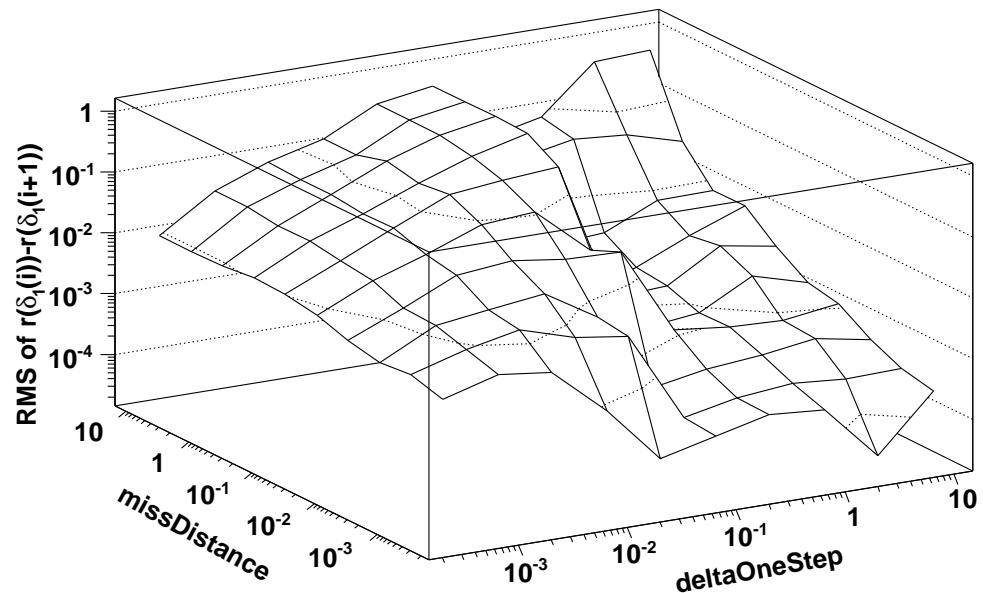
Fig. 2: Error on position vs tracking parameters miss distance and deltaOneStep.
