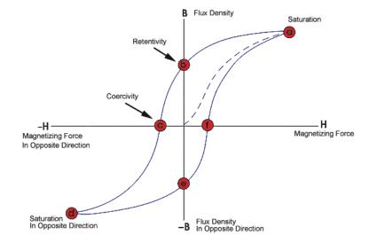
•In order to degauss the circuits, we excite them with plus/minus the operationally used maximum current followed by an amplitude decay
