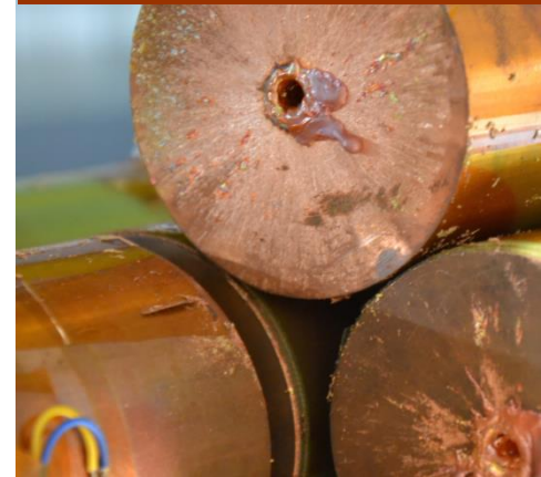
Damage of a beam with an energy of 2 MJ
