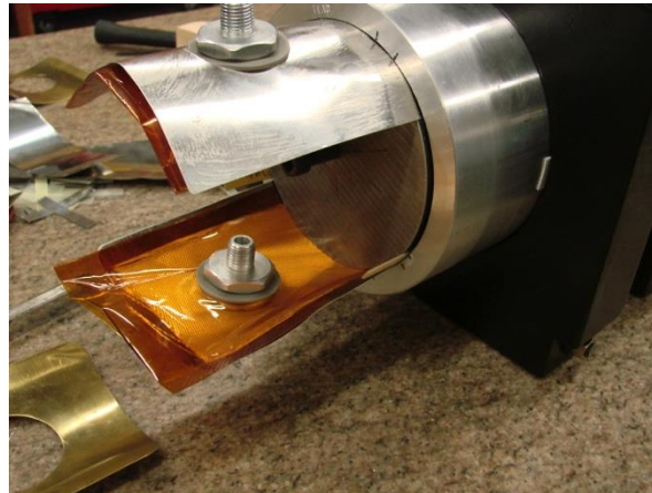
Shims and Bag Inserted Between Layers
