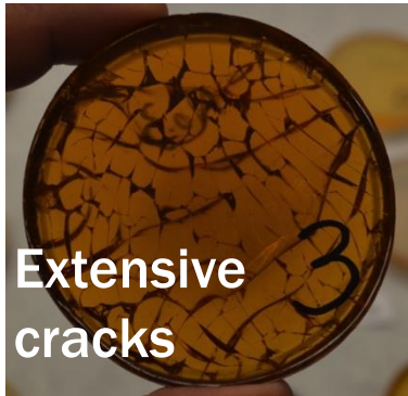
CCTD-101K after one thermal cycle to 77 K
