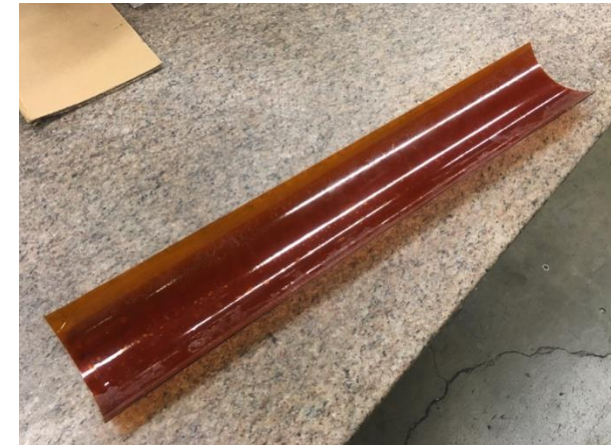
Kapton Bag Filled with Cured Epoxy was Extracted
