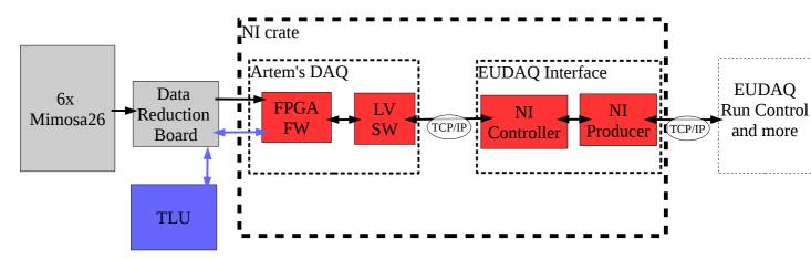
In red: current (Artem's) integration → to be replaced In blue: TLU communication Trigger-Data-Handshake
