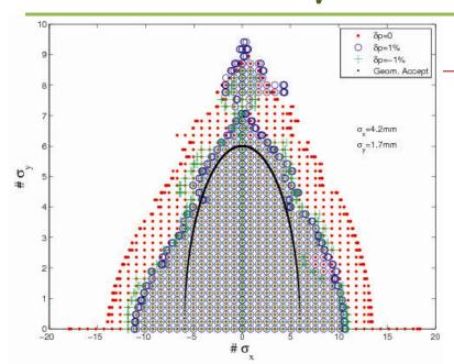
On and off-momentum dynamic aperture for  $\delta p = 0$  (red), 1% (green) and -1% (blue). The geometrical acceptance is also shown.
