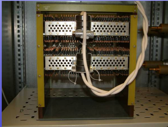
The 25 \Omega PFL : rather compact (2 coax cable // type RG 220)
