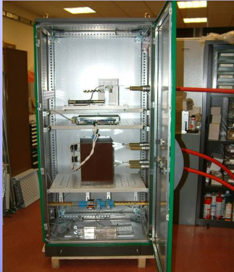
The 25 \Omega PFL : rather compact (2 coax cable // type RG 220)
