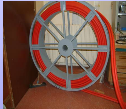
The 25 \Omega PFL : rather compact (2 coax cable // type RG 220)
