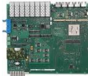
Digital Board (Xilinx V2P FPGA)
