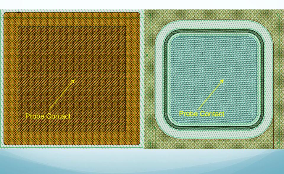
MOS1: Oxide Thickness: 4 microns Capacitance: 2.16 nanoFarad (.863 nF/cm^2) MOS2: Oxide Thickness: 5 microns Capacitance: 2.5 nanoFarad (.690 nF/cm^2)
