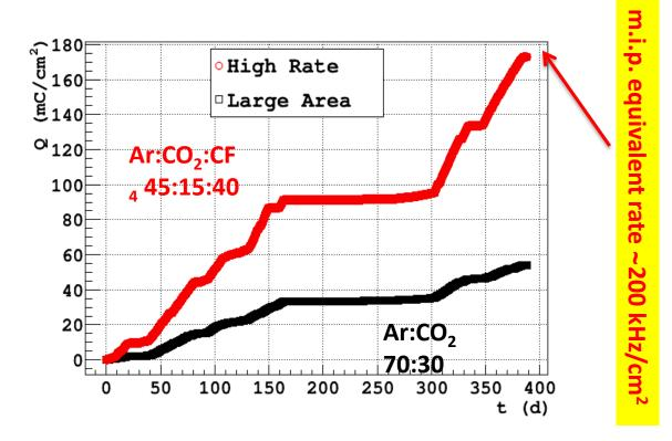
The ageing effects on DLC is under study at the GIF++ by irradiating different  $\mu$ -RWELL prototypes operated at a gain of ~4000 .
