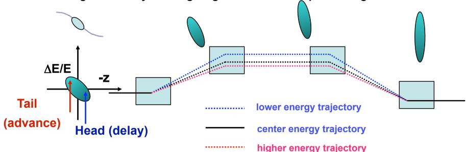
☐ To compress a bunch longitudinally, trajectory in dispersive region must be shorter for tail of the bunch than it is for the head.
