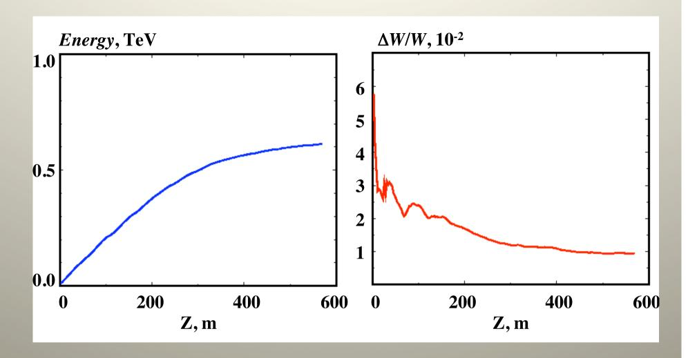
A 1 TeV proton beam, compressed to 100 microns but with 10% momentum spread, would allow to create a 600 GeV electron beam.
