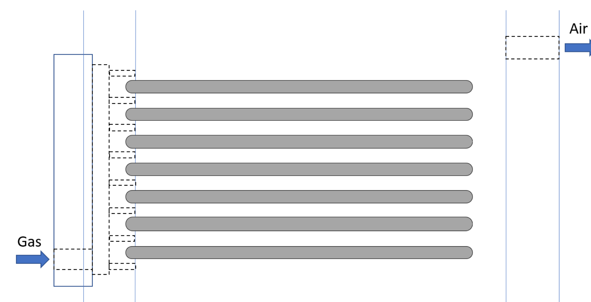
Figure 3: The gas flow schematic for the full chamber. Gas enters through a hole in the gas manifold and flows to all gaps between plates via smaller gas inlets in the back face. Air can then be pushed out through the gas outlet on the front face.
