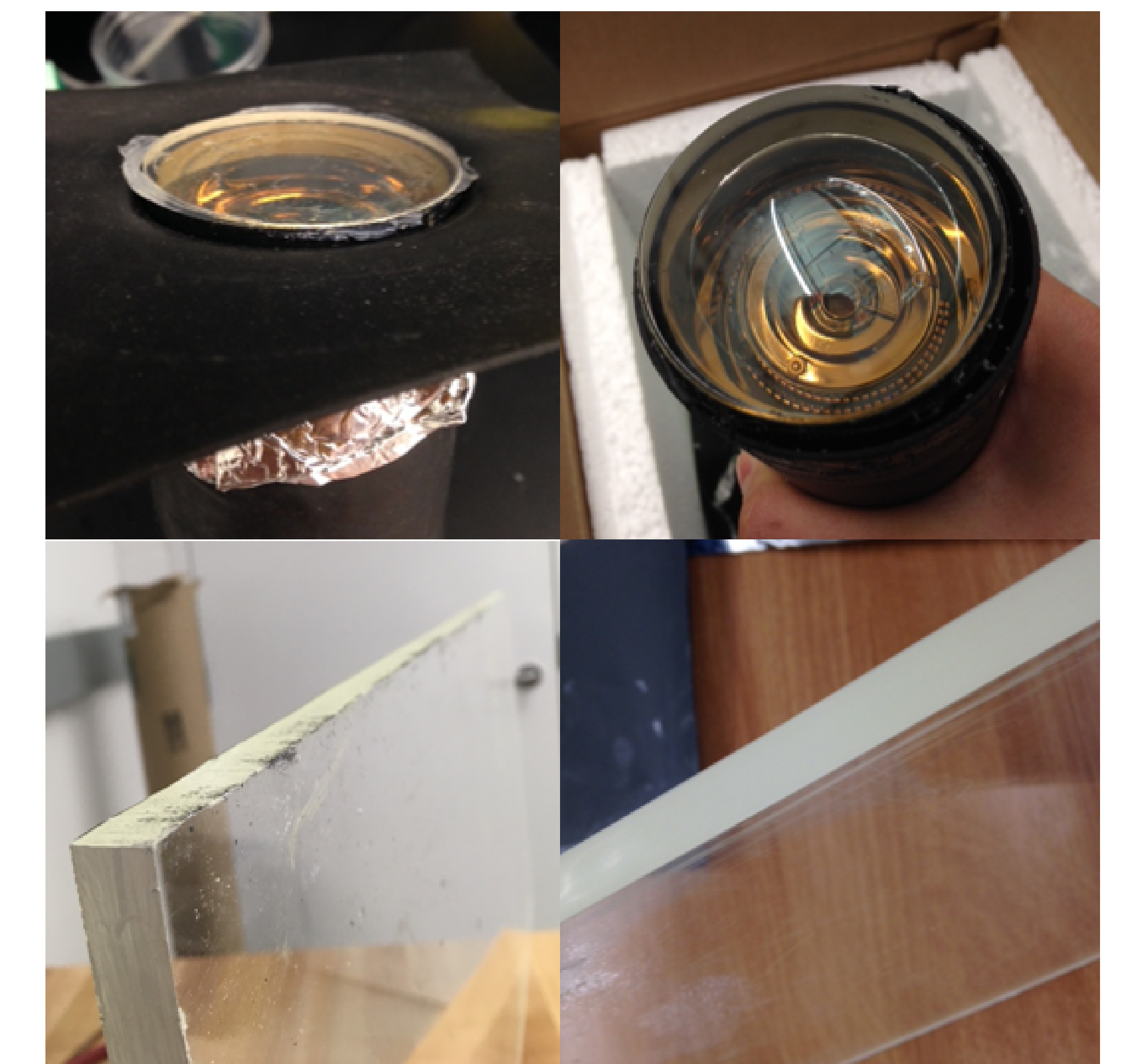
Figure 5: (Left-to-right) Visible ring of rubber glue on PMT lens before scraping; after scraping; scintillator, before polishing; after polishing with 600, 800, and 1200 grit sandpaper.
