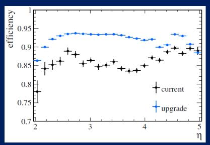
→ improved tracking performance at upgrade luminosity with Fibre Tracker
