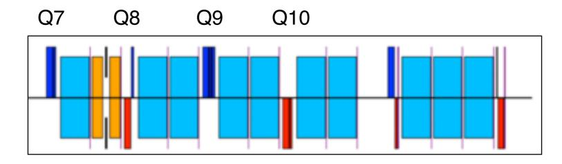
Without upgrade, peak losses in dipoles coil for **0.2h lifetime** are 21 mW/cm³ (protons) and 58.2 mW/cm³ (lead ions)
