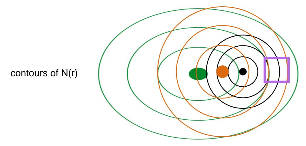
Time of arrival across shower front, "curvature" of two-dimensional N(x,y), .. should distinguish these possibilities and allow position of shower core to be fitted. Then you can fit shower shape with MATHUSLA sampled area.
