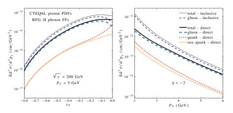
Plot above shows cross-section for direct-photon components (thick lines) as well inclusive (direct+fragmentation, thin lines) photons.
