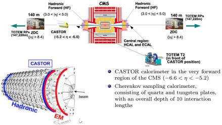
This talk covers results on energy measurements using CASTOR & DPS WW production
