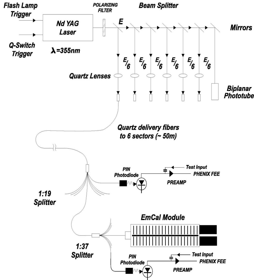
A Nd:YAG laser fires between physics events. Its light is split multiple times and carried to the calorimeter by fibers. Leaking fibers go through quad-tower modules, the leaked light imitates the shower depth profile of a 1 GeV EM shower.
