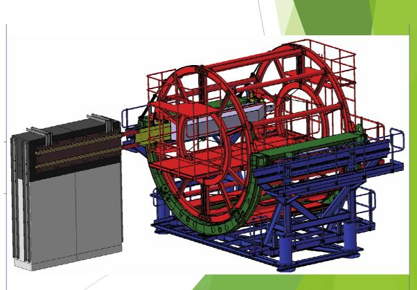
End cap calorimeter assembly
