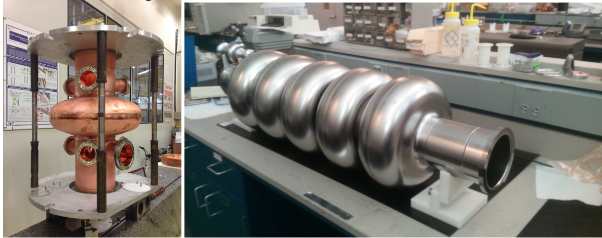
Figure 3.16: Left: A single-cell 400-MHz Nb/Cu cavity built for the LHC. Similar cavities will be used for the Z pole operation of FCC-ee. Right: A prototype FCC five-cell 802 MHz bulk-Nb cavity, for tt operation, fabricated and tested at Jefferson Lab [290].
