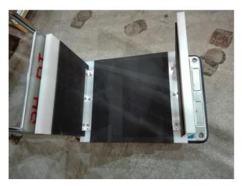
Concrete : For high energy neutrons Polyethylene : for low energy neutrons Boron-carbid : to stop thermal neutrons
