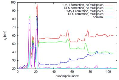
DFS in the Collimation section gives a final vertical emittance  $\Delta \varepsilon_v = 0.7$  nm
