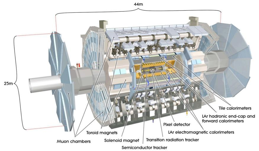
Three main components: inner tracker, electromagnetic (EM) and hadronic (HAD) calorimeters, and muon system
