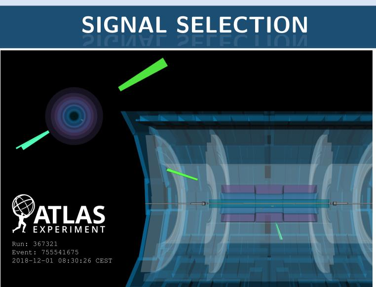
Exactly two photons with  $E_{\rm T} > 2.5$  GeV and  $|\eta| < 2.37$ linvariant diphoton mass  $m_{\gamma\gamma} > 5$  GeV ► Veto extra activity in ID  $\rightarrow$  No tracks with  $p_T > 100$  MeV  $\rightarrow$  No pixel tracks with  $p_T > 50$  MeV and  $|\Delta \eta(\gamma, track)| < 0.5$ Back-to-back topology  $ightarrow p_T^{\gamma\gamma} < 1$  GeV (2 GeV for
