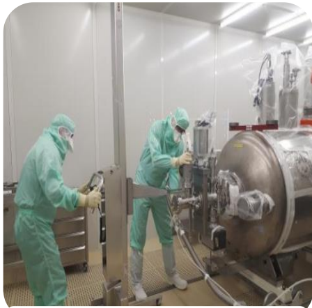
Assembly of new pumping crosses
