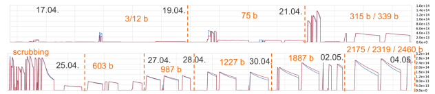
Figure 1: Intensity Ramp up 2018: the beam intensity in B1 and B2 is shown in blue and red, respectively. The stored number of bunches is indicated in orange and the issuing of a checklist by a dashed vertical orange line. The date of the check-list is given in black next to the dashed vertical line.
