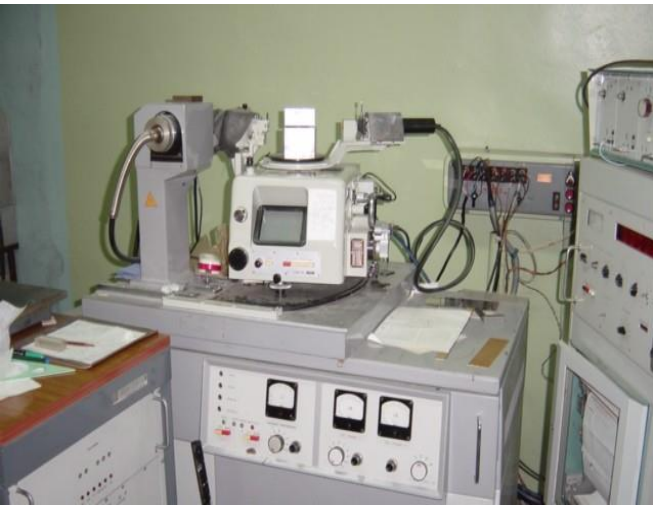
Crystal orienting with X-rays
